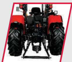
REAR LIFTING CAPACITY OF 5511 lbs & 6613 lbs (OPTIONAL)
