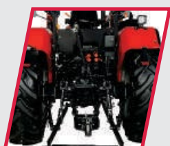
ENHANCED 3- POINT LINKAGES WITH QUICK ATTACH & TELESCOPIC TYPE OPTIONS
